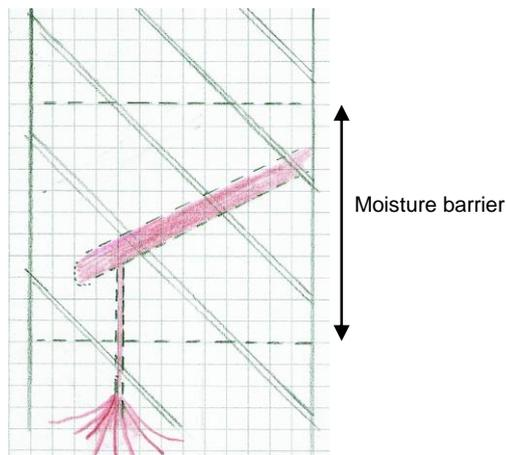
Figure 2: uncontrolled leakage of injection fluid outside the planned moisture barrier
