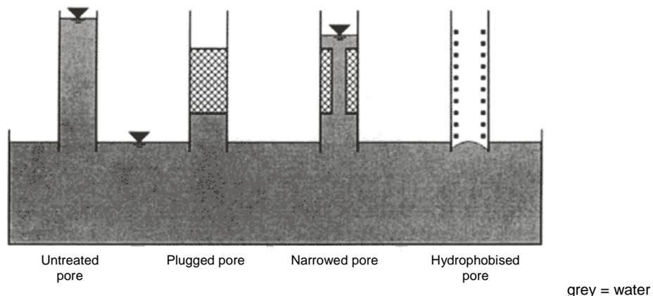
Figure 1: the working mechanism of injection agents, source: /2/
