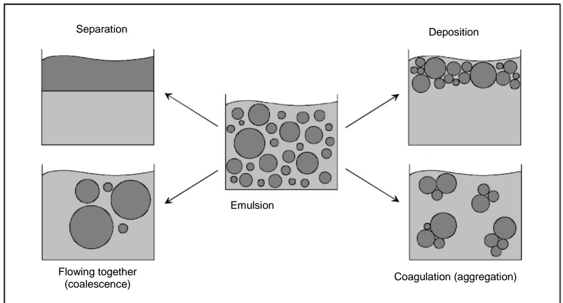
Figure 3: the possible reactions of an emulsion if this is not (sufficiently) stable
