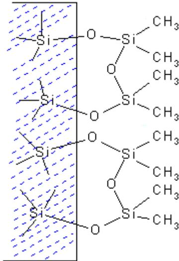
figure 4: attachment of silicone resin to the base, source: /17/
